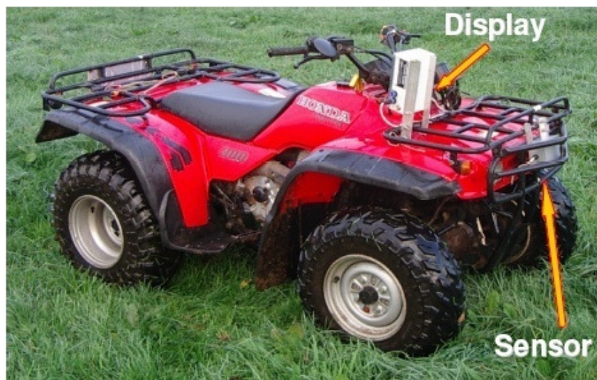
Figure 3. Automatic Pasture Reader mounted to an ATV
