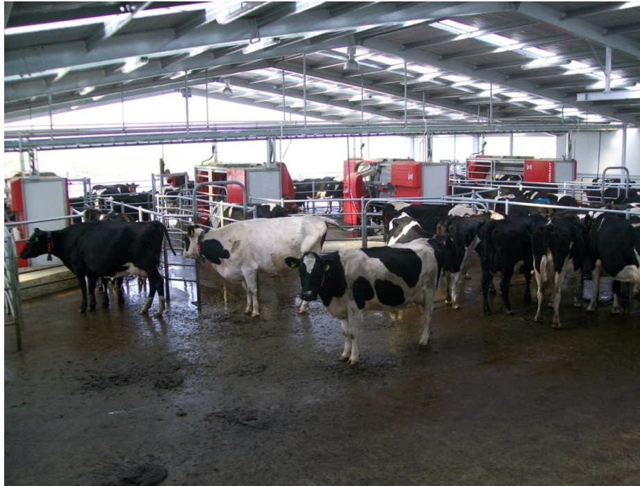
Figure 2. The Overgaauw farm dairy layout showing four Lely A3 with cows in the premilking waiting area (foreground) and the post milking exit area (furtherest from AMS)
