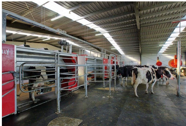
Figure 5. Inside the dairy showing four AMS and cows in the waiting area
